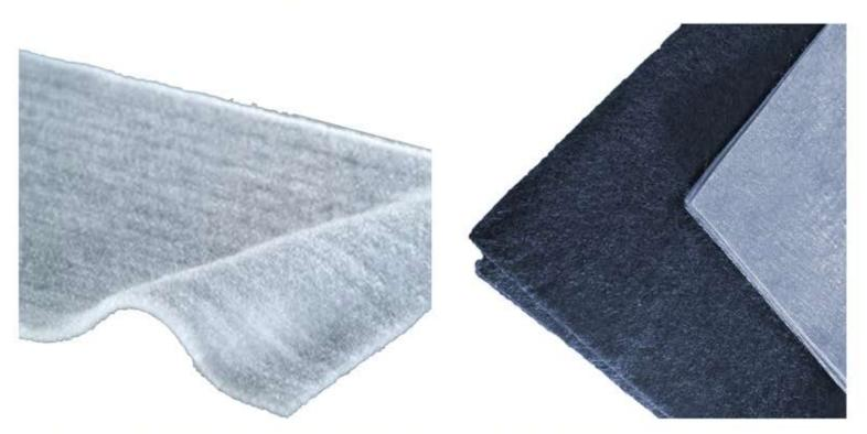
Geotextiles are permeable fabrics which, when used in association with soil, have the ability to separate, filter, reinforce, protect, or drain. Typically made from polypropylene or polyester, geotextile fabrics come in three basic forms: woven (resembling mail bag sacking), needle punched (resembling felt), or heat bonded (resembling ironed felt
